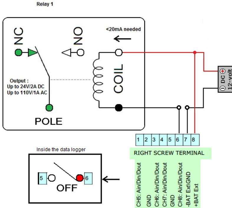
When the conditions are satisfied, the switch closes, and current flows through the relay's coil inductor. However, the relay must be small, ie its coil must be activated via a current lower than 20mA (the max current the logger's digital output can supply).
